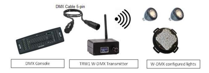
Lights configured with wireless W-DMX control capability can be set up to operate in a DMX512 universe with a DMX console by using a W-DMX (Wireless Solutions) transmitter (such as the LUXAPEL **TRW1**) which will broadcast signals from the DMX control console.
