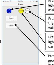
Press SCAN + SETUP to seek unpaired lights and jump to connect page for assignment of groups and info
